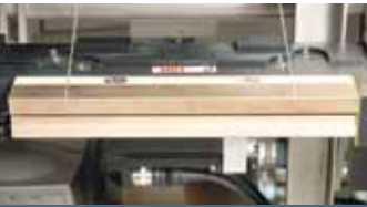
Easy open cereal style sealing jaws
